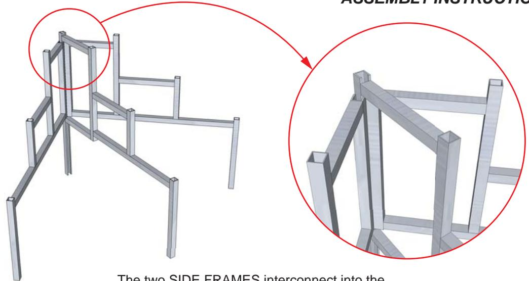
The two SIDE FRAMES interconnect into the CENTER FRAME. The back vertical of the SIDE FRAMES hook into the back vertical of the CENTER FRAME.
