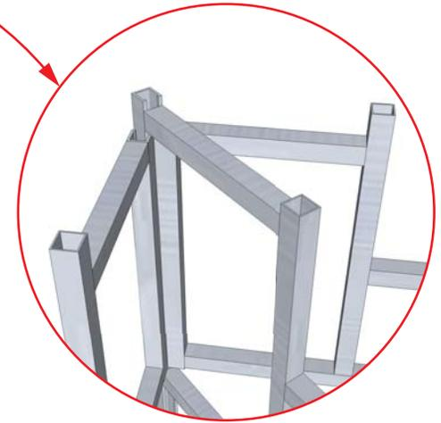
The two SIDE FRAMES interconnect into the CENTER FRAME. The back vertical of the SIDE FRAMES hook into the back vertical of the CENTER FRAME.
